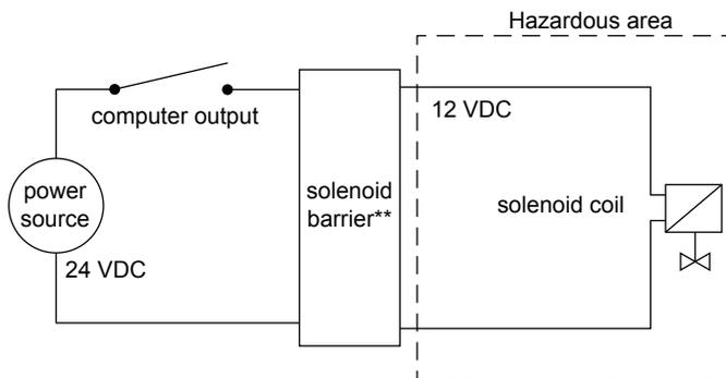
\*\* Use of an intrinsically safe 24 VDC solenoid barrier with internal impedance, or end-to-end resistance, of 250 to 305 ohms required for proper operation of StoneL's intrinsically safe solenoids.
