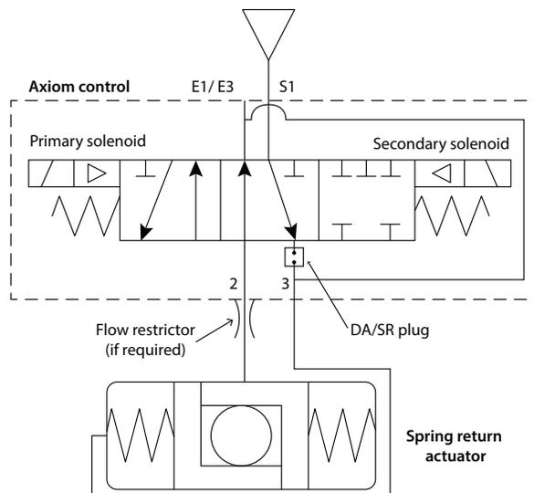
Fig. 5 Expeditor pneumatic valve on double-acting actuator
